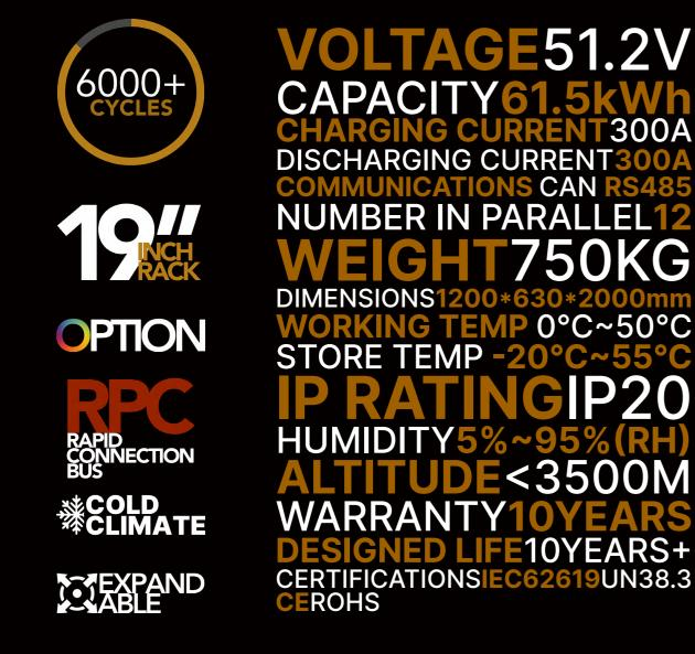
The Voltsmile Raid12 Energy Storage System, the ultimate high-capacity solution for your energy storage needs. This state-of-the-art system houses up to twelve RPC Mark2 lithium iron battery packs, delivering a combined power of 61.5kWh. Equipped with built-in three-phase inverters, the Voltsmile Raid12 ensures ease of installation and reliable power for both residential and commercial applications.
