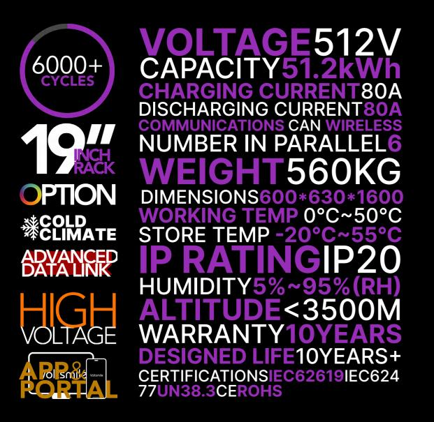
The Voltsmile C512 High Voltage Lithium Iron Energy Storage System, a state-of-the-art solution designed to meet the energy demands of large homes, small offices, and small businesses. With an impressive voltage of 512V and a substantial capacity of 51.2kWh, the Voltsmile C512 ensures reliable and efficient power storage, making it the ideal choice for high-capacity energy needs.
